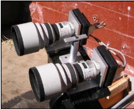
The XO Project uses this inexpensive "telescope" (a pair of 200-mm f/1.8 telephoto camera lenses) to monitor the brightnesses of tens of thousands of stars every night. The lenses are attached to CCDs, which can measure slight dips in star brightnesses that reveal a transiting planet. The telescope is on the summit of Haleakala, a volcano on Maui. Courtesy
