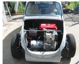
100% biodiesel generator in area of original trunk
