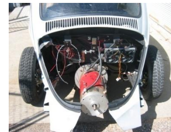
NetGain Warp 9 motor connected to original transmission
