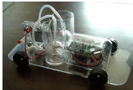
Reversible fuel cell, water electrolysis
